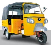
Rear Engine Passenger 3+1 500 kg Payload Capacity
