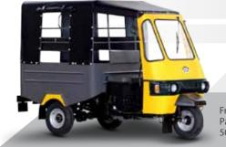
Front Engine Passenger 6+1 500 kg Payload Capacity
