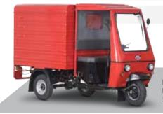
Front Engine Delivery Van 500 kg Payload Capacity
