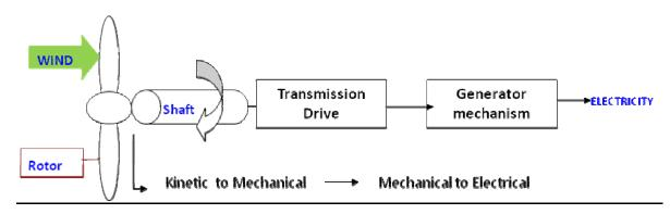
The above flow depicts the principle and mechanism of generating power from wind, Thereafter, the power generated by wind turbines is conditioned properly so as to feed the local grid as shown in below picture.
